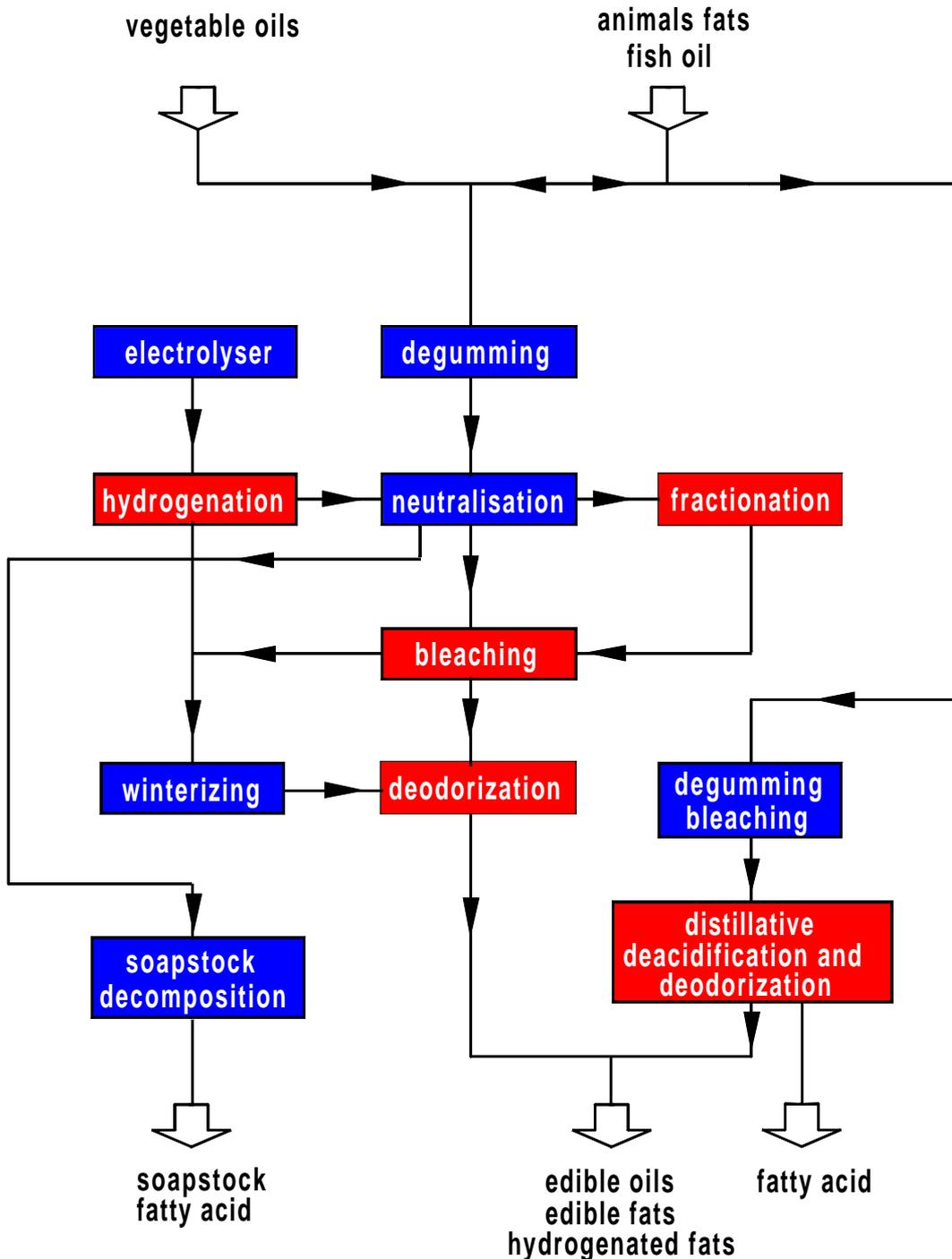
This picture shows the various process stages in the processing of edible oil.
