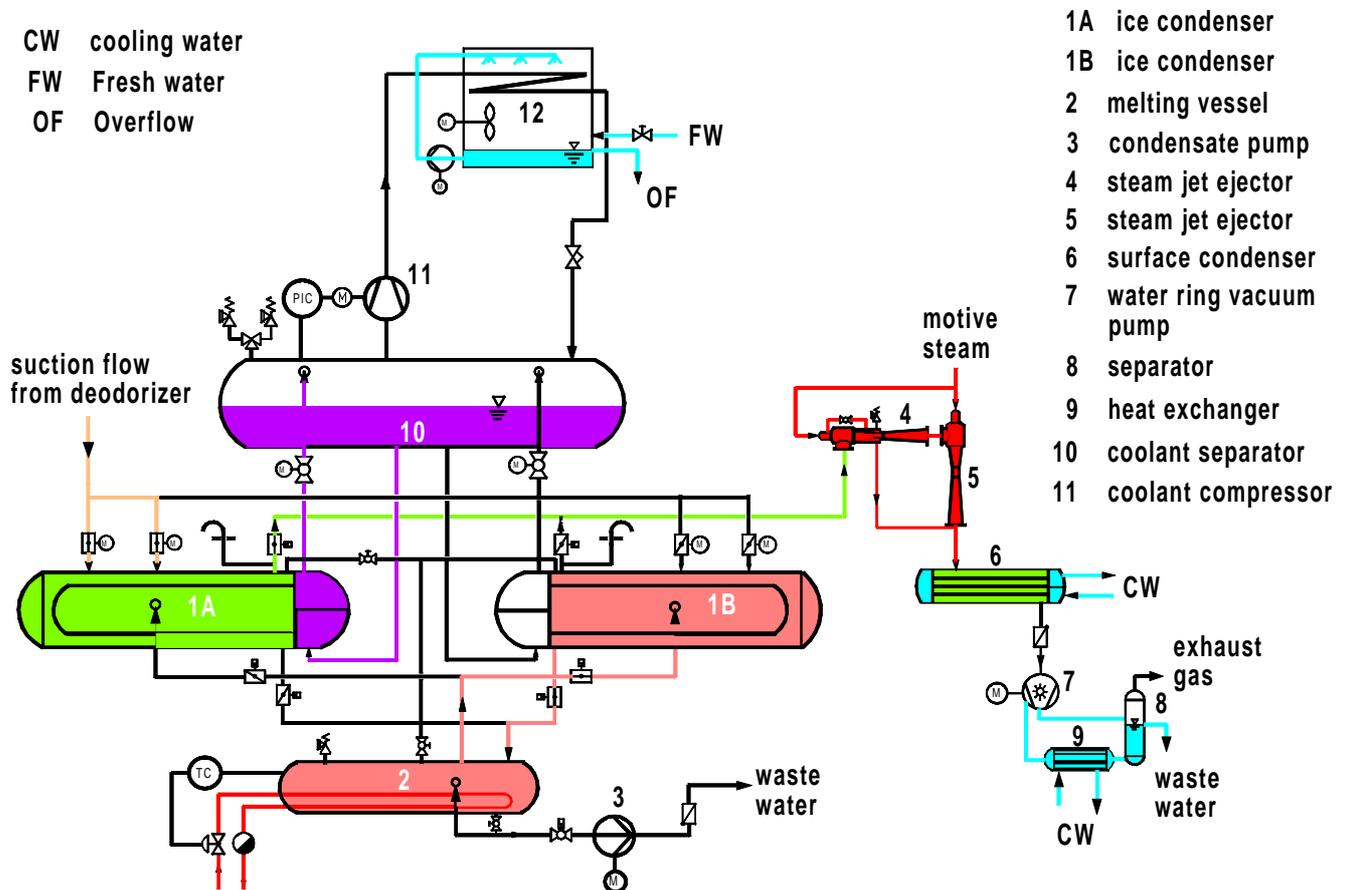
Following the idea to condense the stripping steam at the lowest possible temperature and pressure leads to a system where the stripping steam can be condensed at the process working pressure of the column. In case this pressure is below 6 mbar, water vapour condenses into the ice phase.
