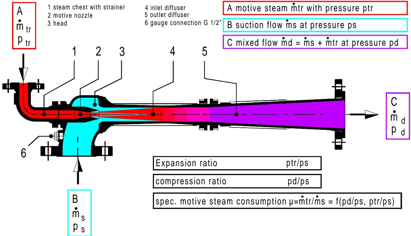
The compression attainable from the suction nozzle to the outlet nozzle is, dependent on the motive pressure, the specific motive steam consumption, and finally on the internal geometry of the ejector.
