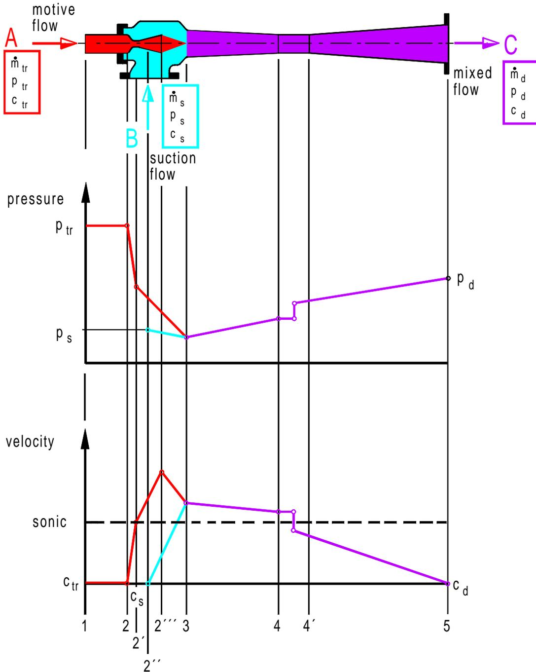
The motive flow enters the motive nozzle with a fixed pressure and velocity. It is not possible to transfer the high energy of the motive flow directly to the suction flow.
