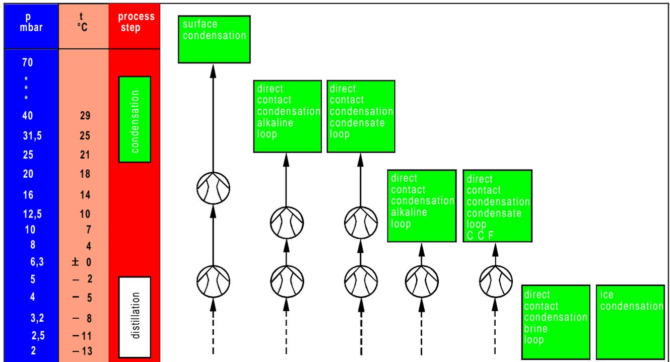
In the realisation of this separation numerous systems have been developed which are shown in the picture above:
